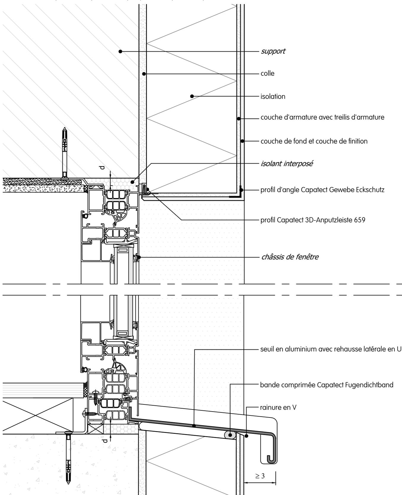
Isolant interposé  $R \geq 1.5 \text{ m}^2 \text{ K/W}$ .
